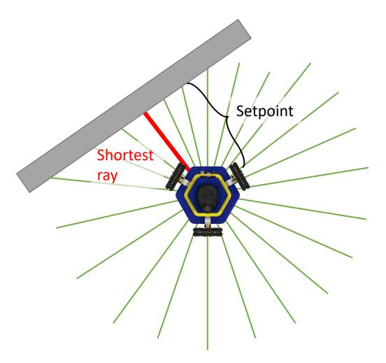
**Goal:** Write a controller so that the robot maintains a distance to the *nearest* wall.
