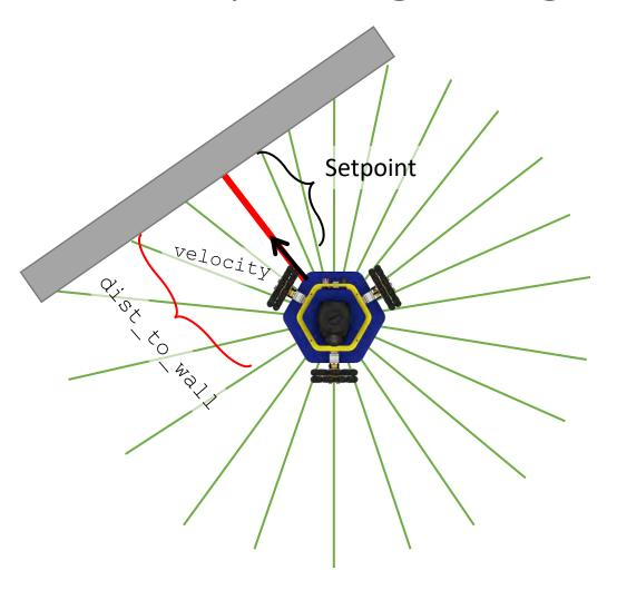
We can use the same controller (bangbang or P-control) as last week. But this time, we'll drive in the direction of the shortest ray.
