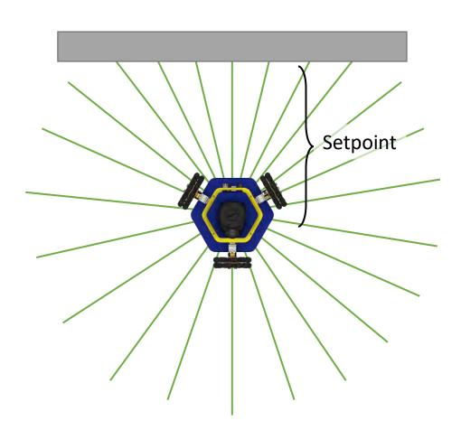
Goal: Write a controller so that the robot drives towards the wall and stops a certain distance from the wall.
