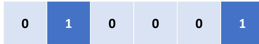
The distance transform is the distance from each free cell (0) to the nearest occupied cell (1). We can write down the answer by inspection:
