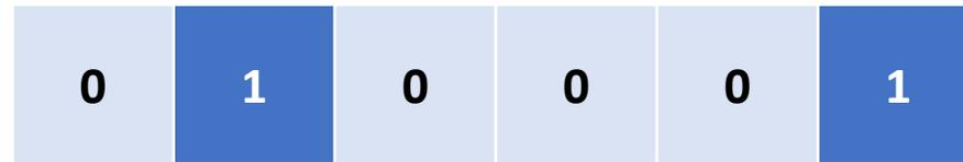
The distance transform is the distance from each free cell (0) to the nearest occupied cell (1). We can write down the answer by inspection:
